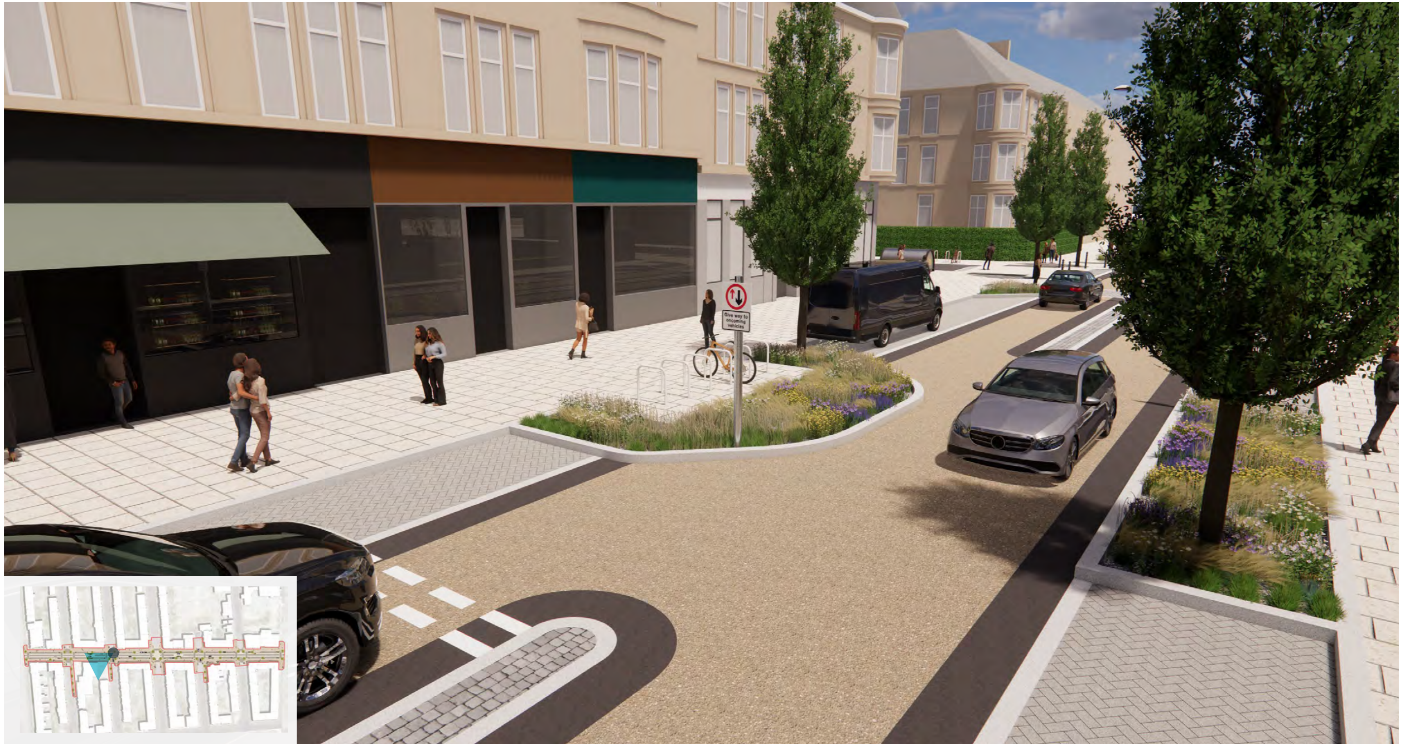
Figure 28: 3D Visualisation showing proposed rain garde, street tree planting, priority giveway traffic calming measure and integrated parking
