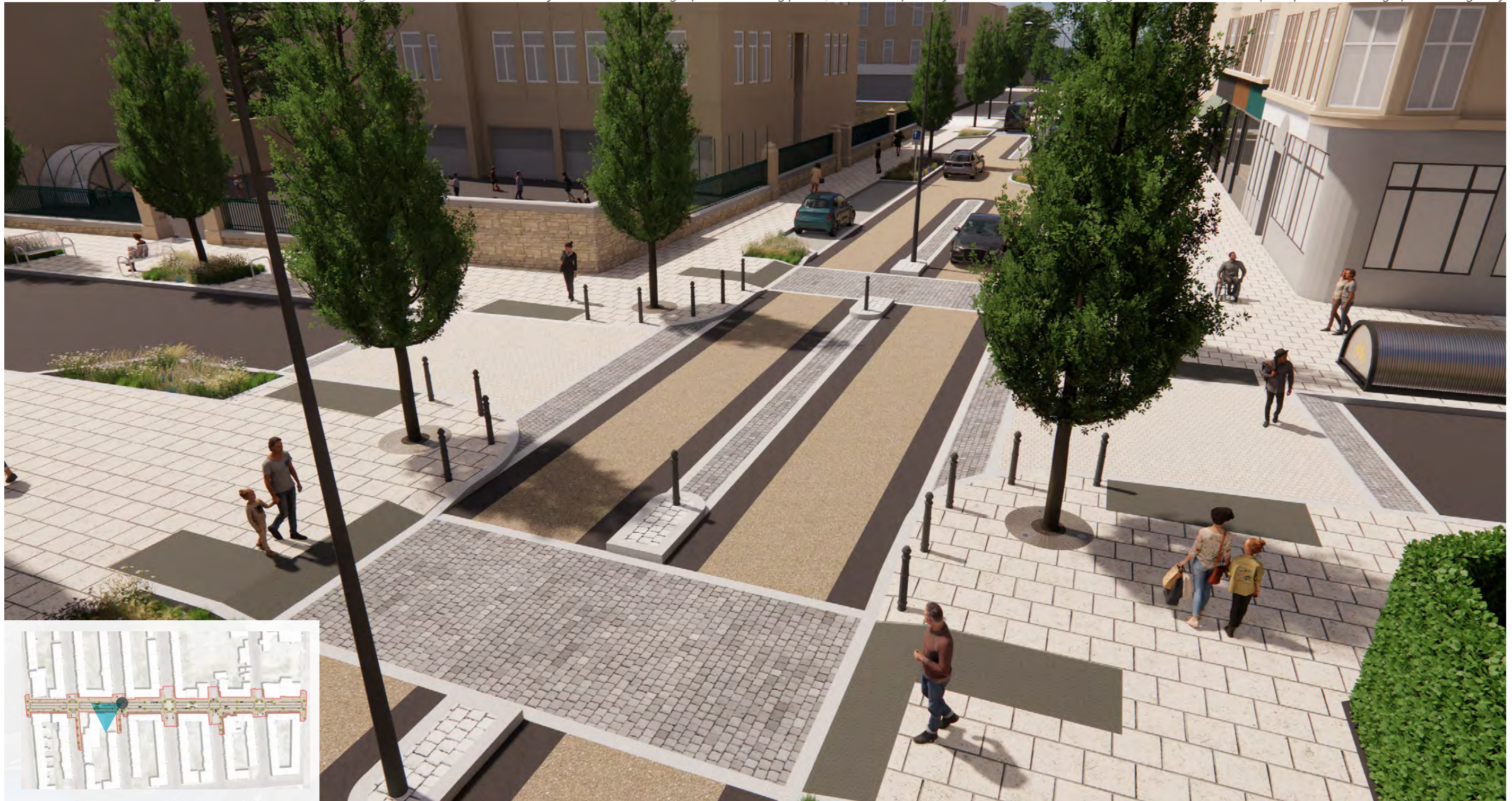
Figure 27: 3D Visualisation looking towards Pollokshields Primary School and showing informal crossing points, continuous footways and central median along Albert Drive to create a perceptual narrowing of the carriageway
