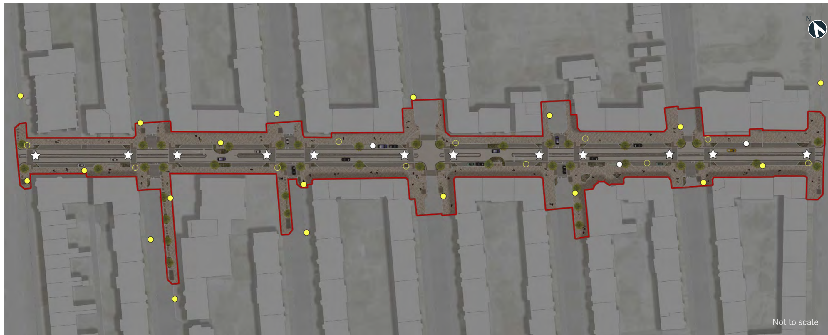
Figure 30: Plan showing existing and proposed street and feature lighting along Albert Drive
