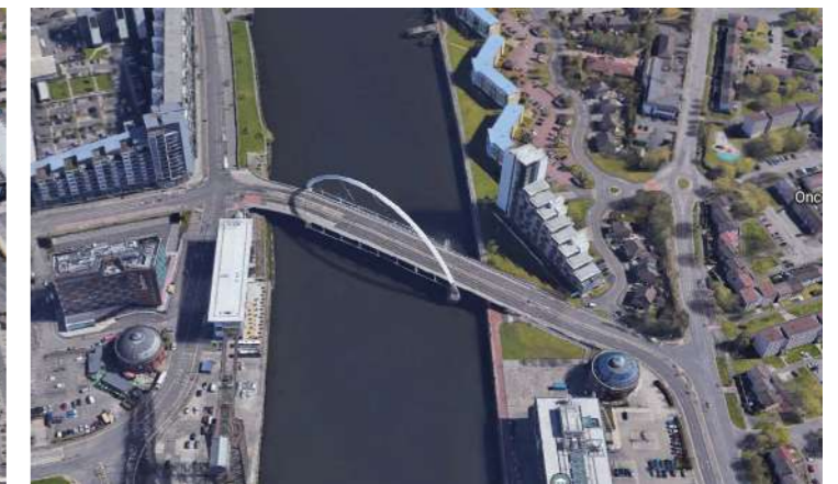
8 - Bridge between the Riverfront hotel area/Plantation. Most of the Space on the bridge is taken up by the 4 traffic lanes (16m wide) leaving pavements under 2m wide to either side. During Cop26 the bridge became completely car and bus free, and this has been noted in Commonplace as a positive thing by residents.
