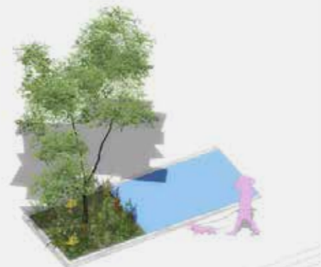
LEVEL TREE PLANTER WITH RAISED CONCRETE SURFACE PLANTER 1000 X 1000MM RAISED CONCRETE 1000 X 2000MM
