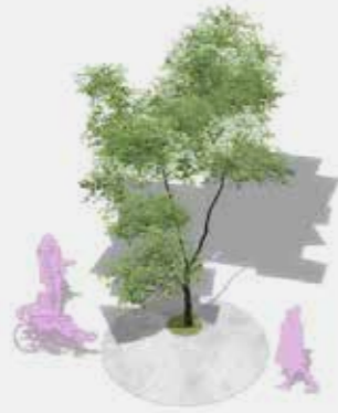
CONCRETE TRANSITIONED PLANTER DIAMETER 12000MM, HEIGHT 800MM
