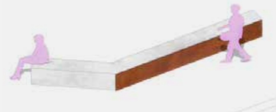
CONCRETE BLOCK WITH CORTEN SHEET
