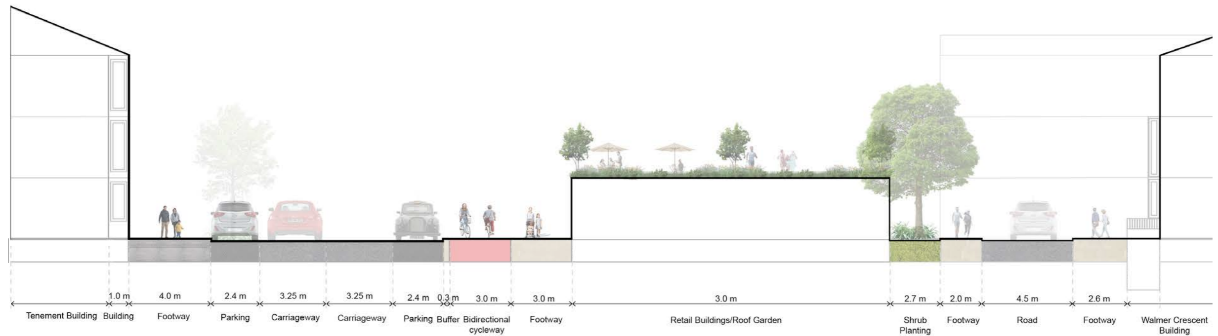
Figure 57. Paisley Road West By Walmer Crescent Section
