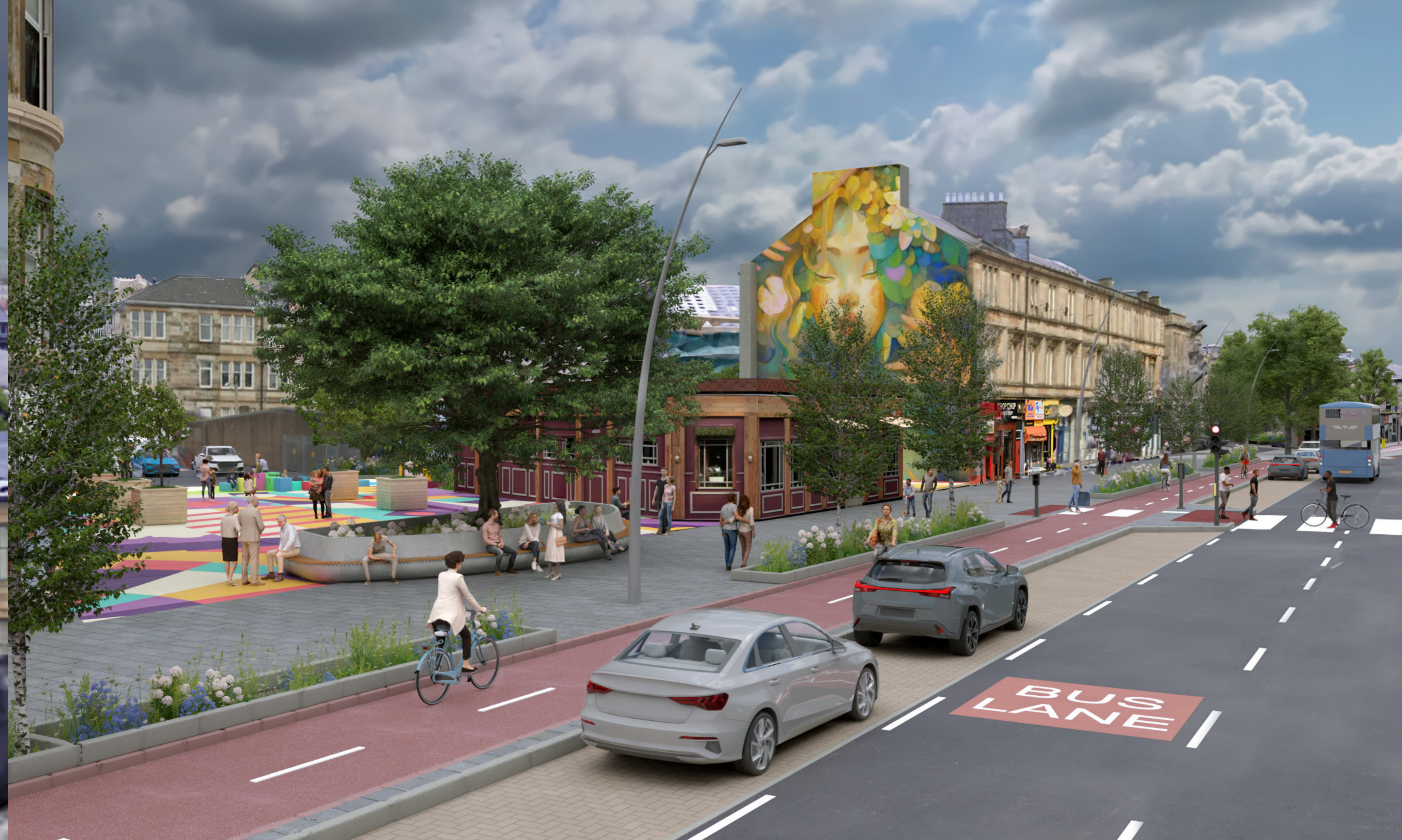
Figure 60. View of Paisley Road West and Elizabeth Street public realm improvements, including high quality paving, segregated bi-directional cycleway, tree planting and rain gardens, street furniture, street art and retained car parking
