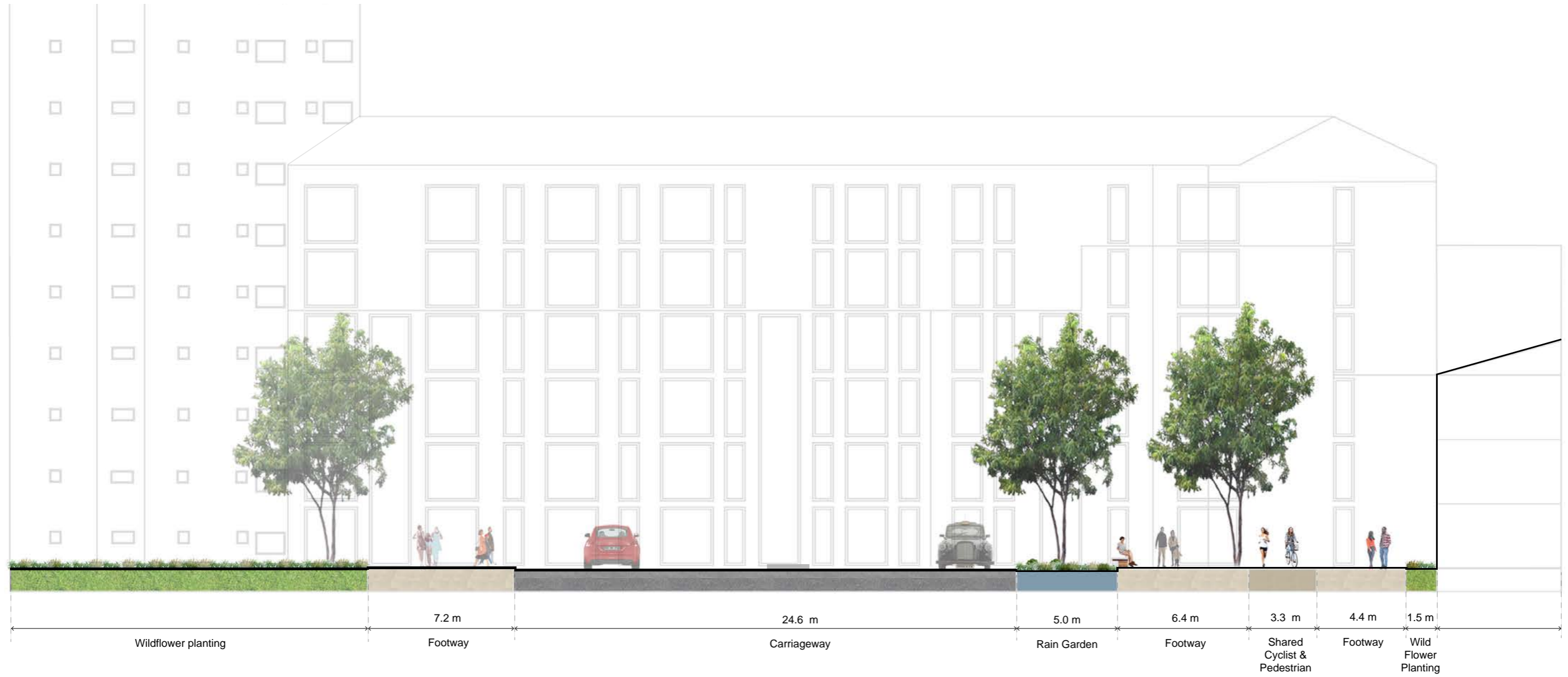
Figure 55. Edmiston Drive Junction Section
