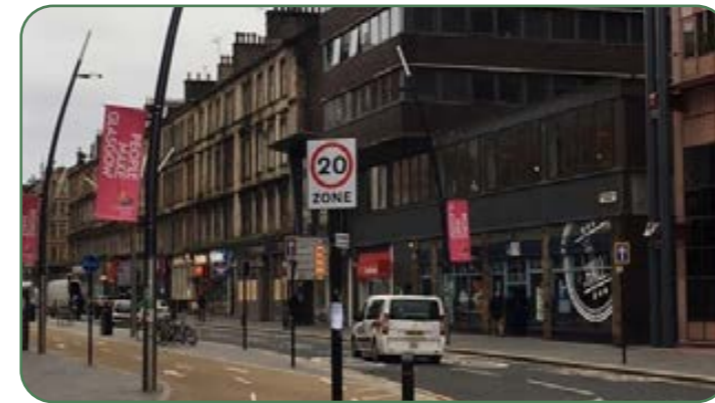
Proposed Street lighting: Black-painted galvanized steel curved lighting columns. Suitable for streetscape
