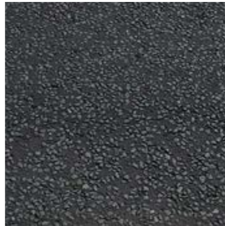
MTL-03 Asphalt with black chips Footways
