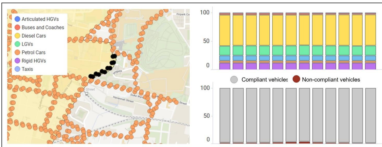
Figure 21: The contribution to modelled NOx concentrations from different vehicle types, at roadside points along High Street.
