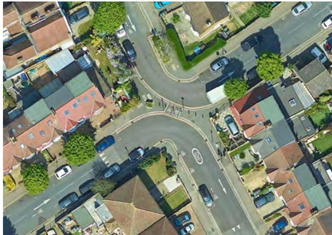
Figure 4.26: after image of aerial view after a modal filter has been added to cross section.
