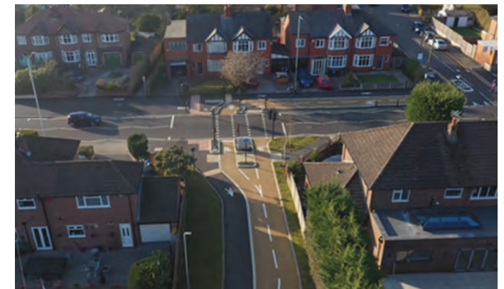
Figure 4.48: Aerial image of crossing which has protected cycleway crossing alongside pedestrian crossing.
