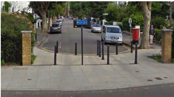
Figure 4.20: Example of a side street modal filter in London where people can walk or cycle across but not drive.
