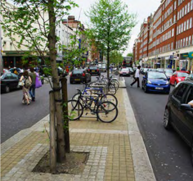
Figure 4.70: Cycle parking in central median between two trees so does not clutter pedestrian spaces.
