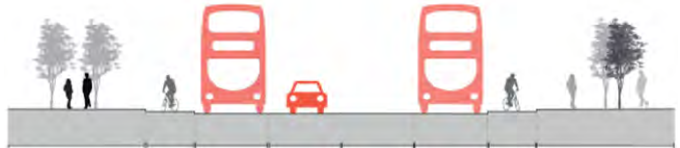
Figure 4.8: Generic example cross section of a wide street catering to different transport modes.
