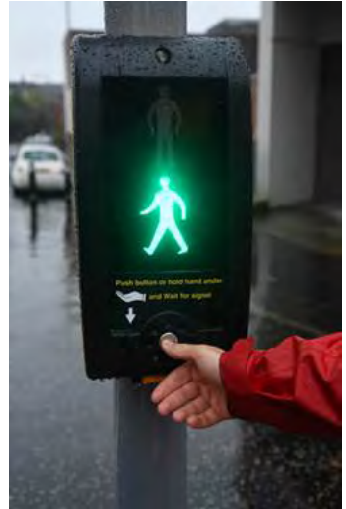
Figure 1.2: Pedestrian light push button, light is currently showing a green safe to cross symbol
