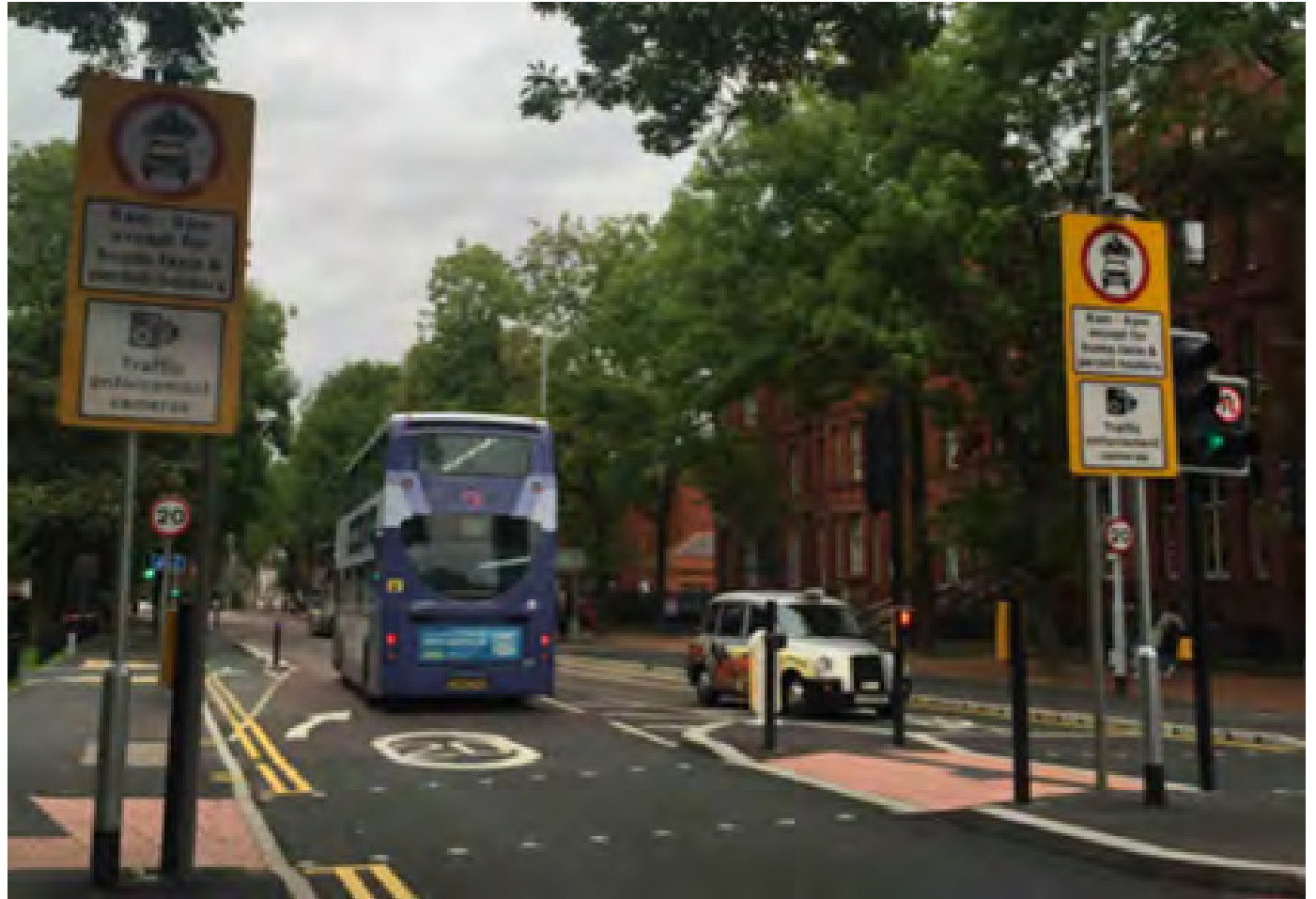
Figure 4.28: Bus gate in Manchester signs in foreground show time of operations and provide information that taxis and permit holders are exempt.
