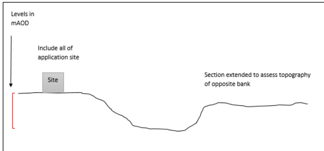
Figure 1. Example of appropriate site cross section.
