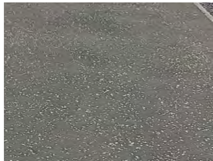
Proposed footway (standard asphalt): Bituminous Macadam
