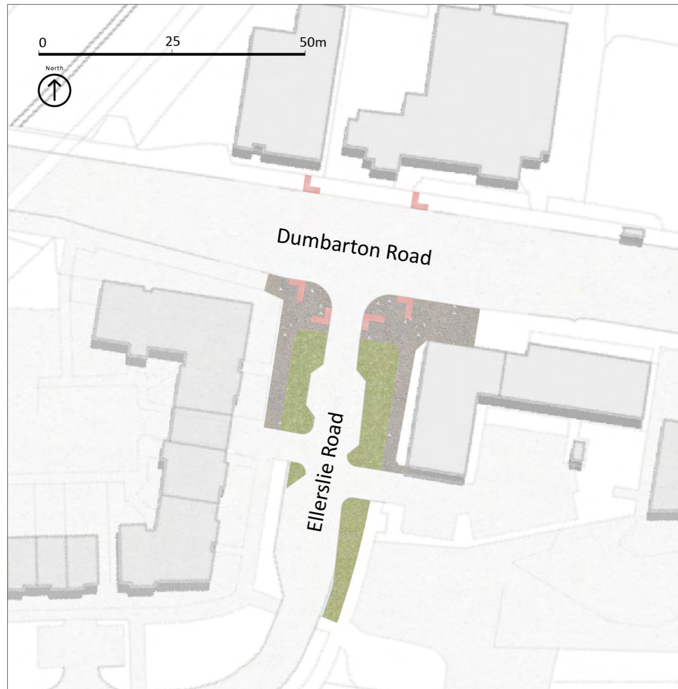
Ellerslie Road - Junction tightening
