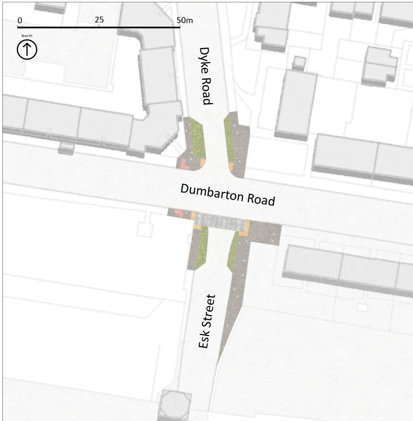
Dyke Road - Junction tightening and Esk Street - Continuous footway
