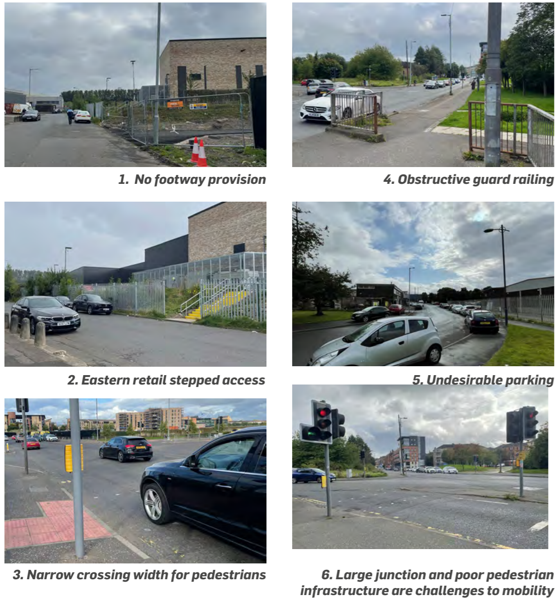
Figure 11: Annotated photos identifying key features/issues on the site
