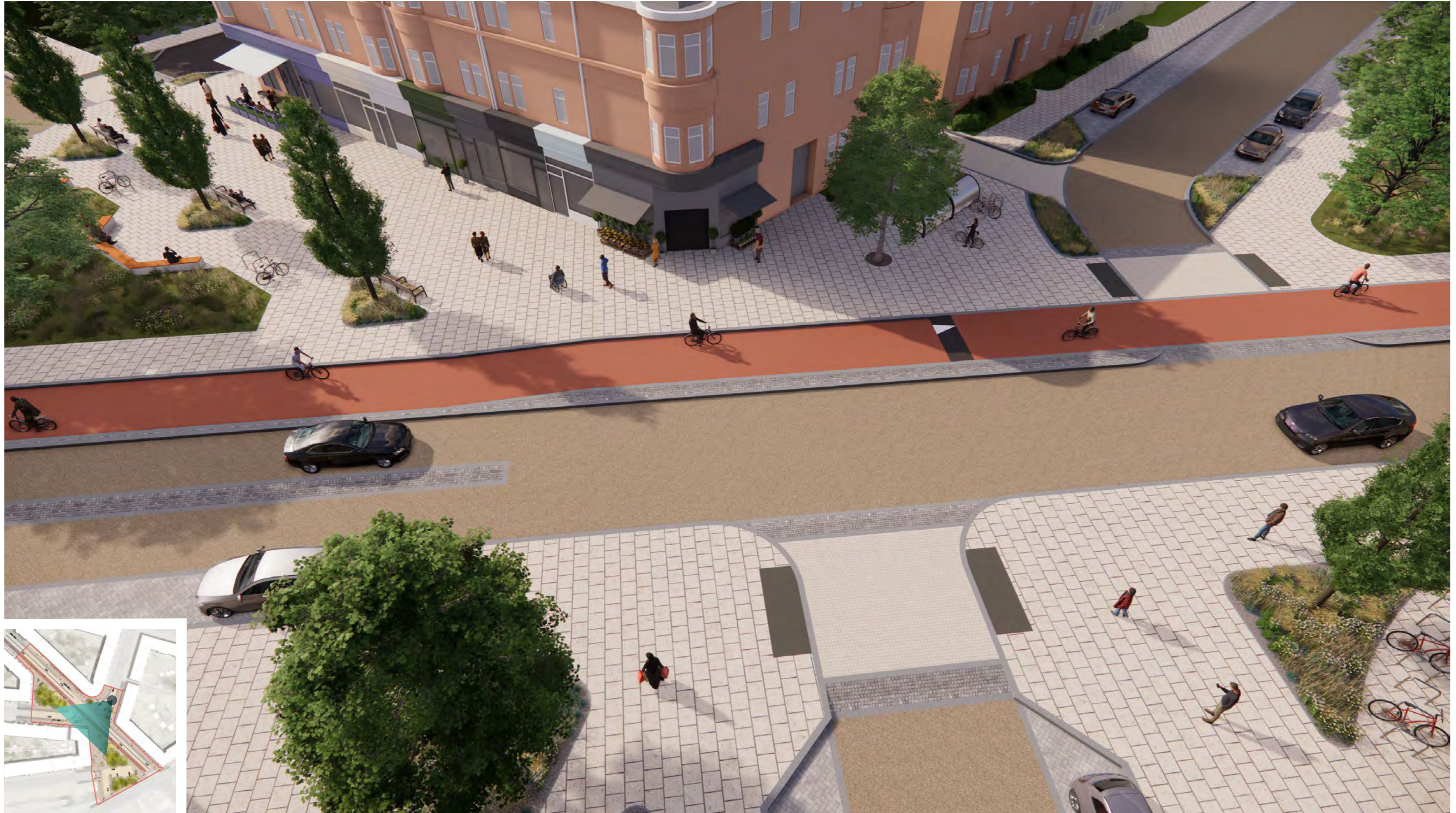
Figure 23: Visualisation showing the creation of new green attractive footway space through the tightening of junctions, narrowing of Nithsdale Road and reallocation of Kildrostan Street
