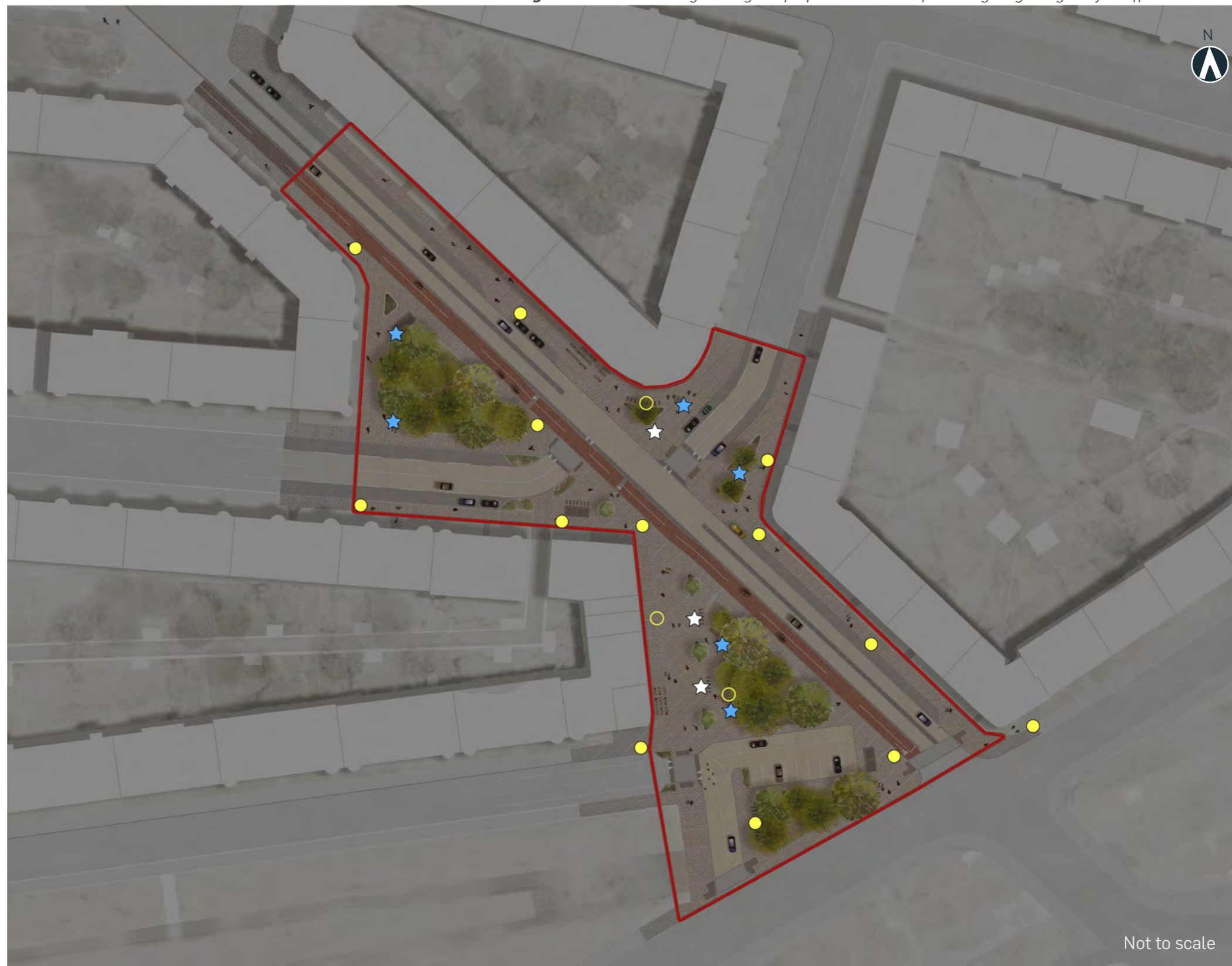
Figure 27: Plan showing existing and proposed street and feature lighting along and just off Nithsdale Road
