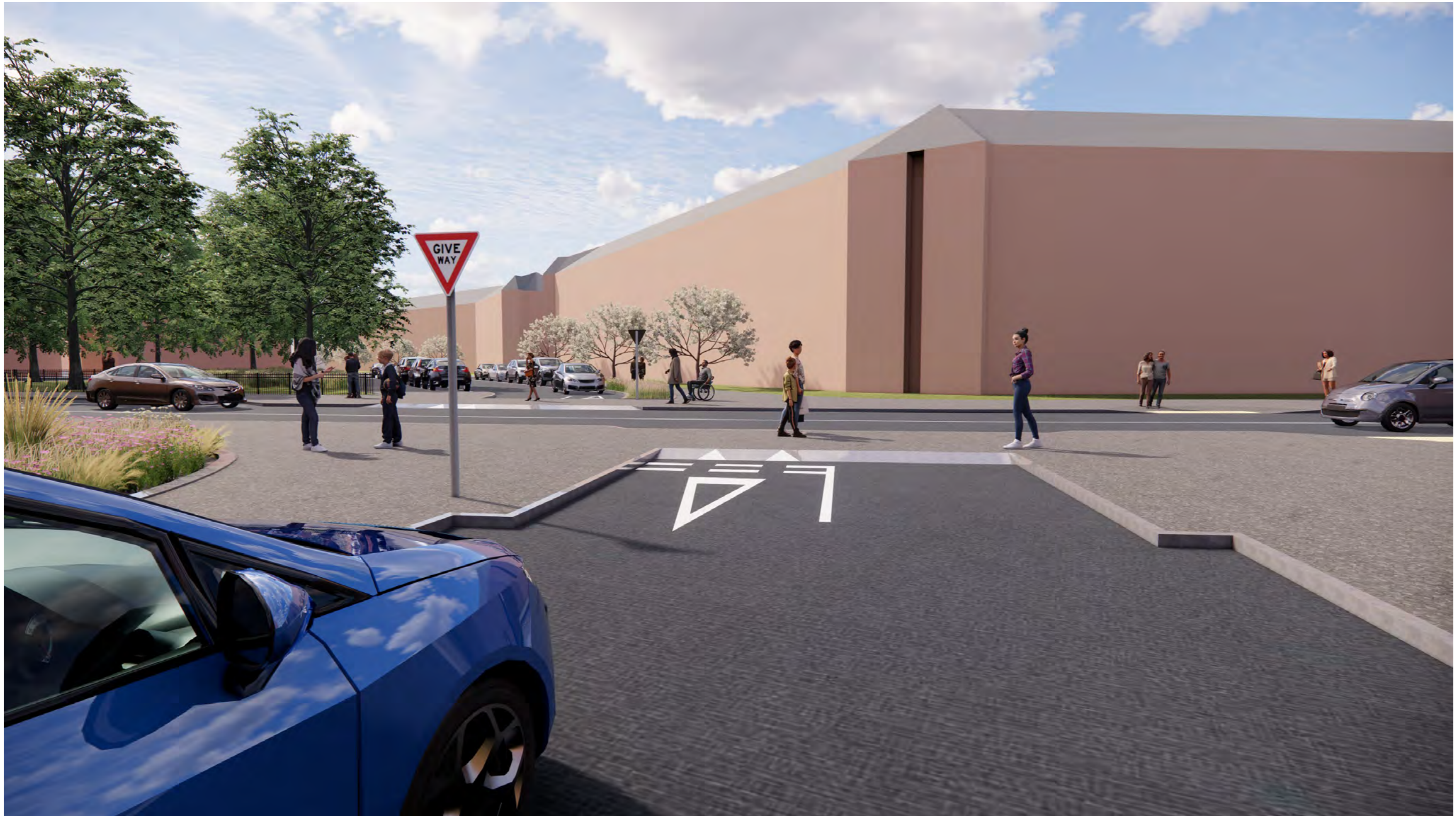
Figure 36: Ground level view visualisation showing an example of continuous footway side street junctions
