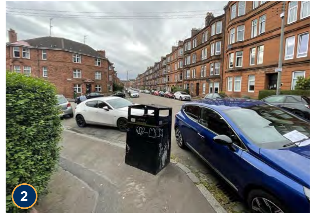
2 Other street furniture obstructions and lack of dropped kerbs / tactile paving.
