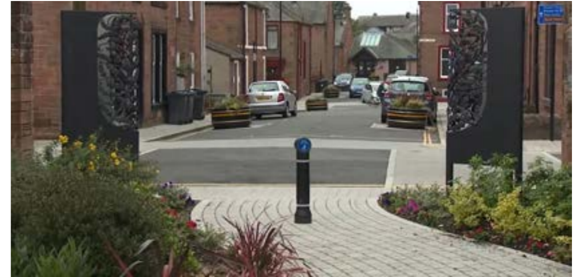
Modal filter with dual access and gateway feature
